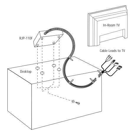
As shown above, install on a desk or cabinet located in a convenient location where connections can be made to the TV display panel. The end user should have easy access to the RJP and AC power outlets should be readily available.
